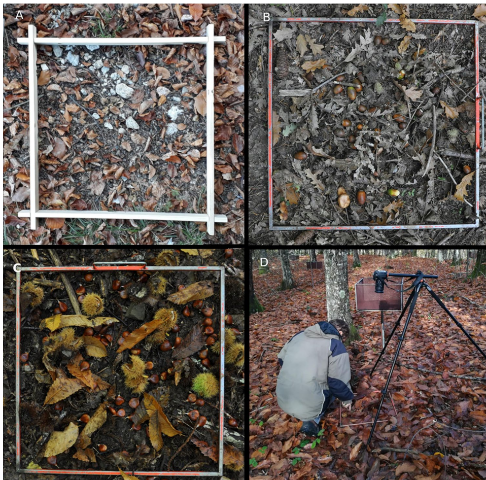
Fig. 2 Examples of seed counting methods used to assess seed production in temperate broad-leaved tree species. A ground quadrat (0.25 m 2 ) placed in beech a , Turkey oak b , chestnut c plots. A downward looking camera to collect quadrat images close to a litter trap d
