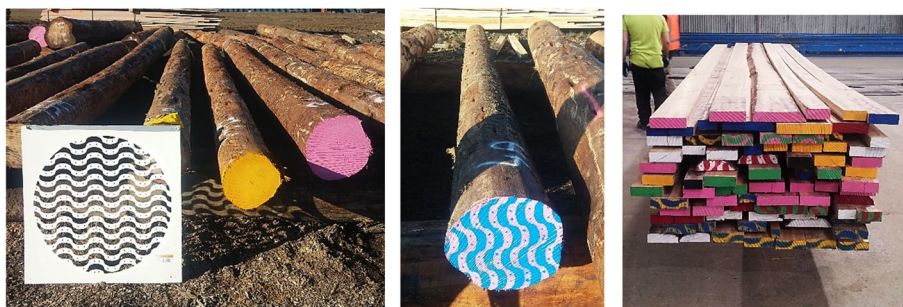
Fig. 1 Pattern used to maintain traceability from logs to sawn boards. Each log end was coloured with a unique colour combination
