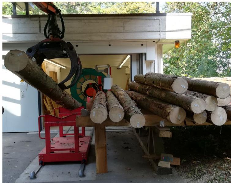
Fig. 8 Installation of a log for CT scanning
